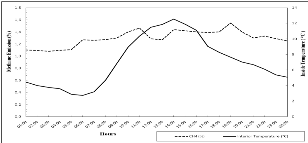
Figure 6. Hourly distribution of averaged methane and interior temperature profile at freestall dairy housing
