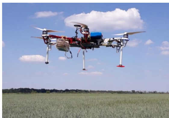
Figure 3. An air sampler mounted on a UAV
